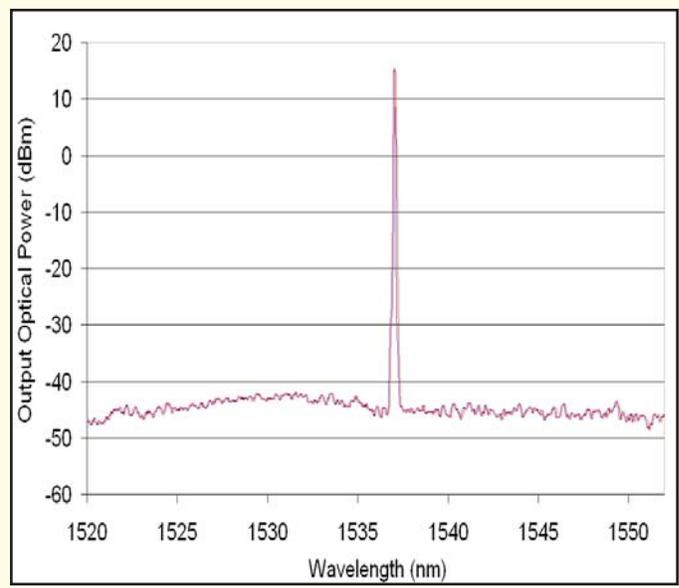
Fig. 3: Stability of the new tunable laser source after idling for one hour at 23°C
