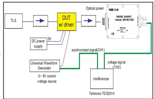
Fig. 4 Testing Method for Tuning Speed Measurement
