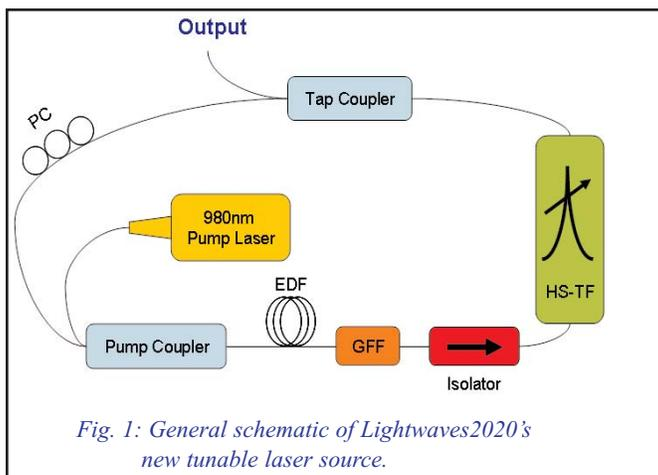
Fig. 1: General schematic of Lightwaves2020's new tunable laser source.
