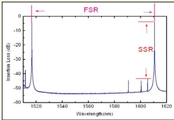
Fig. 2 Transmission Spectrum
