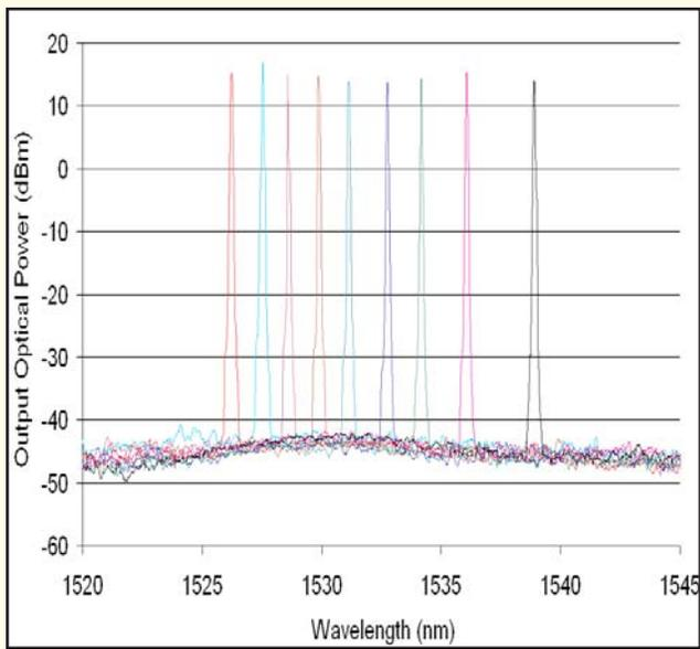
Fig. 2: Example spectral performance of the new tunable laser source
