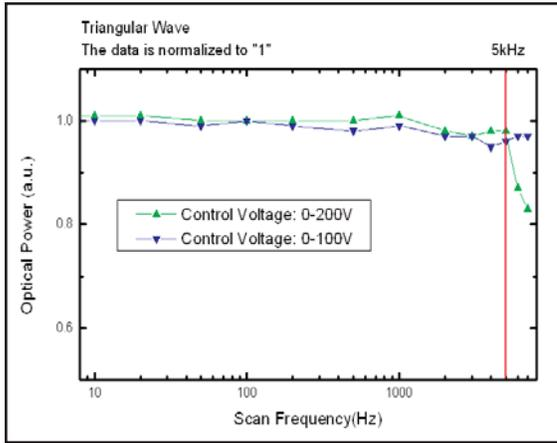
Fig. 5 Optical Power vs. Scan Frequency Curves
