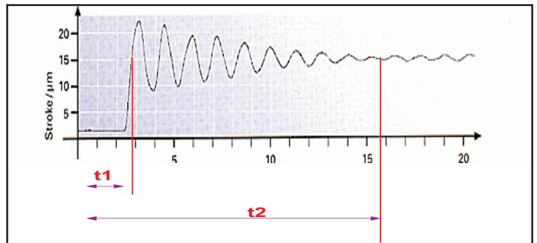
Fig. 6 Typical Response for Piezo-based Actuator
