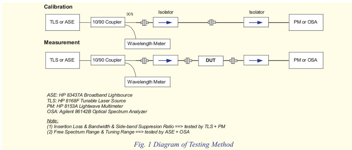
Fig. 1 Diagram of Testing Method
