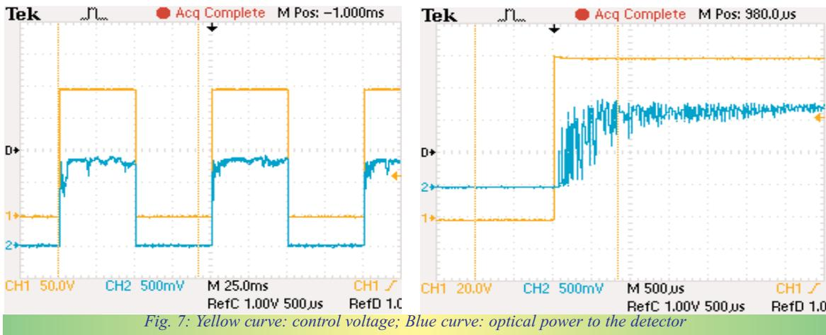
Fig. 7: Yellow curve: control voltage; Blue curve: optical power to the detector
